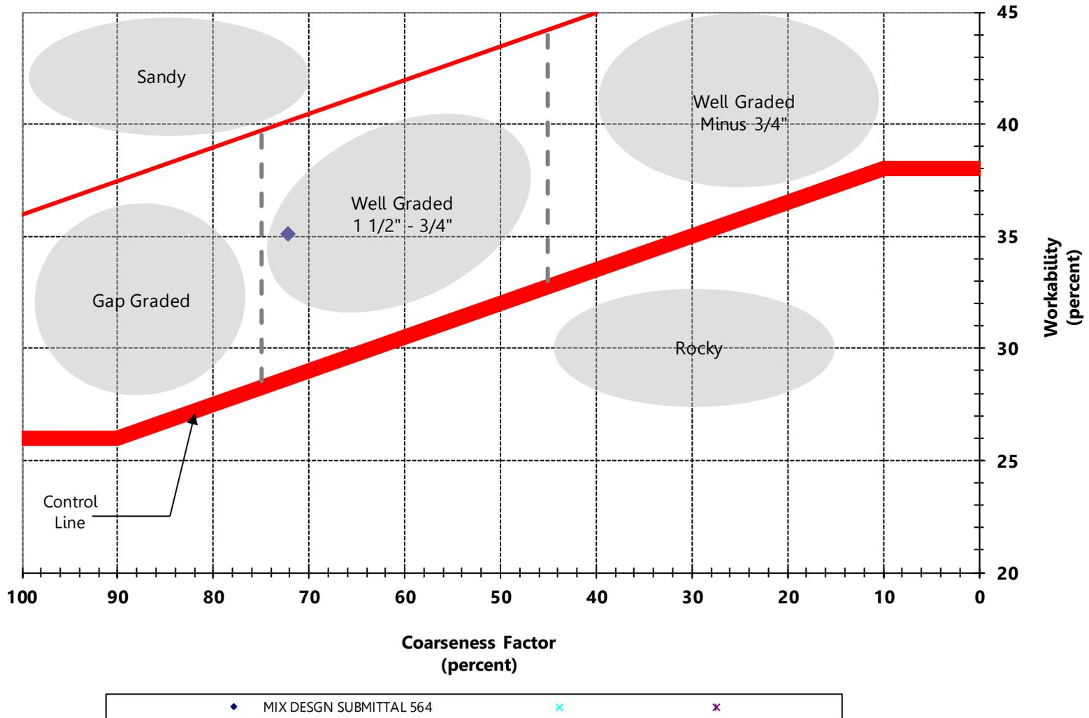
Figure 6. SR-46 Combined Gradation Coarseness and Workability Factors
