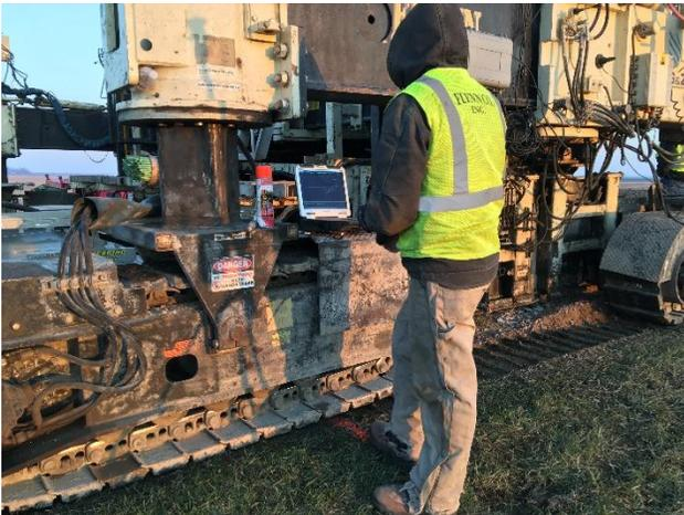
*Figure 5. Flynn Crew Member Observing Real-Time Smoothness Results on the RTP Display*
