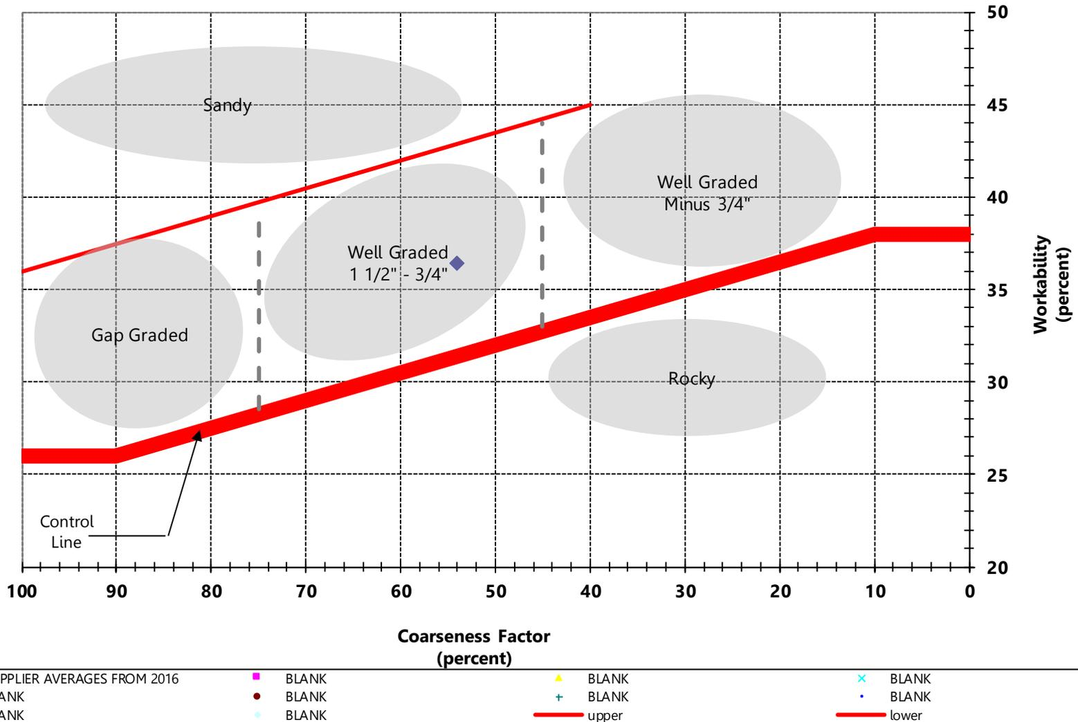
Figure 8. US-20 Combined Gradation Coarseness and Workability Factors
