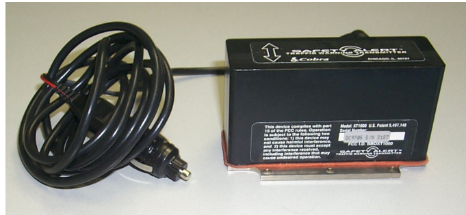
Figure 3-4. K-band drone radar (Fontaine and Hawkins 2001)
