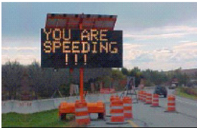
Figure 3-2. Changeable message sign displaying speed message (FHWA 2008)
