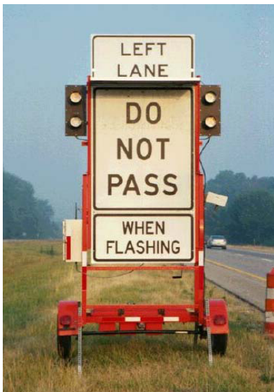
Figure 8-1. Typical dynamic lane merger device (Bushman and Klashinsky 2004)
