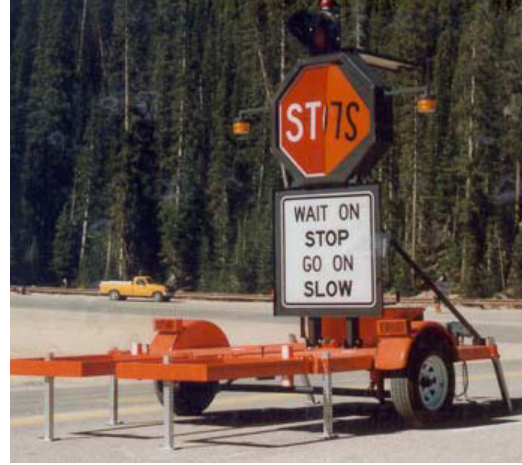
Figure 4-3. AUTOFLAGGER rotating (Mn/DOT 2000)
