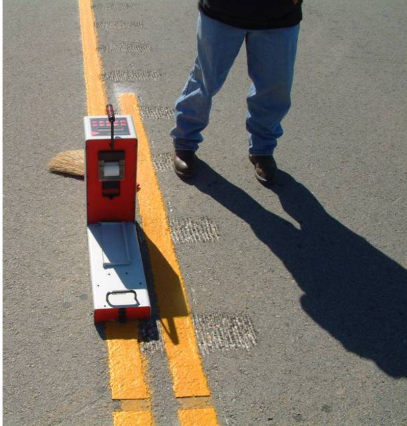
Figure 8. Measuring Rumble Strip Retroreflectivity
