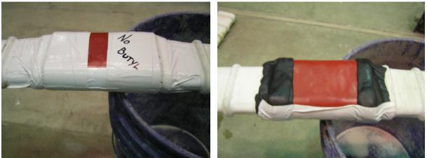
a. Waterproof duct tape b. Butyl rubber and duct tape Figure 3.2. Mockup splice connections for 1 in. x 3 in. P-T duct
