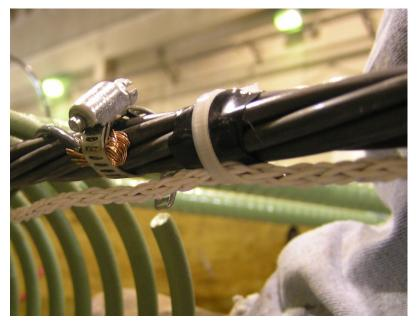
Figure 4.1. Corrosion electrode tied to strand
