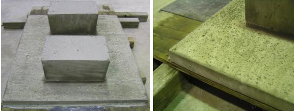
a. Grout filled pockets and haunch b. Close up of grout at haunch Figure 3.1. Stud pocket and haunch mockup after form removal
