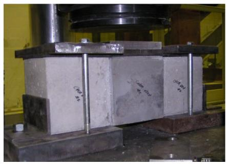
Figure 3.3. Push-out tests for transverse joint surface treatment
