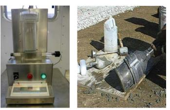
Devices for air content measurement of fresh concrete
