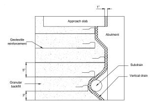
Schematic diagram of drainage details incorporating vertical drain
