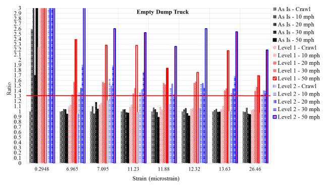
Empty dump truck on short-span pre-stressed concrete girder Bridge 40320
