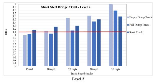
Figure 4.8. DIFs based on largest strain in short-span steel girder Bridge 23370
