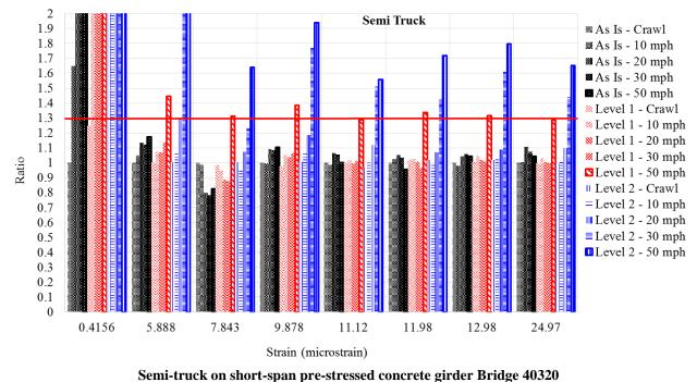
Figure 4.5. DIFs for short-span pre-stressed concrete girder Bridge 40320 under different
