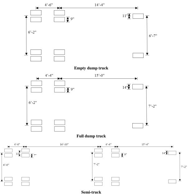
Figure 3.6. Trucks on short-span steel girder Bridge 23370
