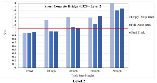
Figure 4.10 DIFs based on largest strain in short-span concrete girder Bridge 40320
