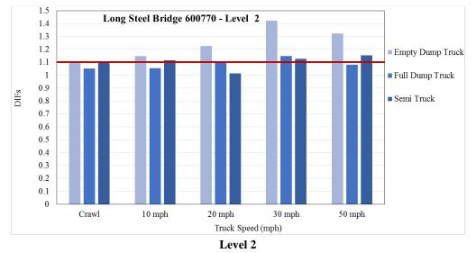
Figure 4.7. DIFs based on largest strain in long-span steel girder Bridge 60770
