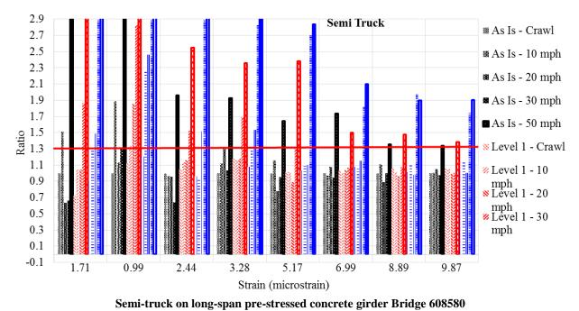
Figure 4.4. DIFs for long-span pre-stressed concrete girder bridge 608580 under different loading scenarios
