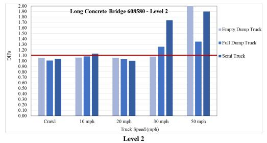
Figure 4.9. DIFs based on largest strain in long-span concrete girder Bridge 608580
