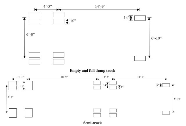
Figure 3.4. Trucks on concrete slab Bridge 30790
