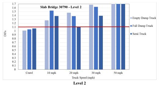
Figure 4.11. DIFs based on largest strain in concrete slab Bridge 30790
