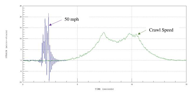
Figure 4.1 Strain time histories for a dump truck crossing a bridge at 50 mph and at crawl speed for the As-is entrance condition
