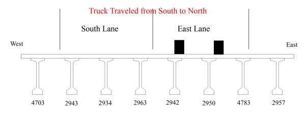
Figure 3.9 Short-span concrete girder Bridge 40320 strain gauge locations and travel lanes
