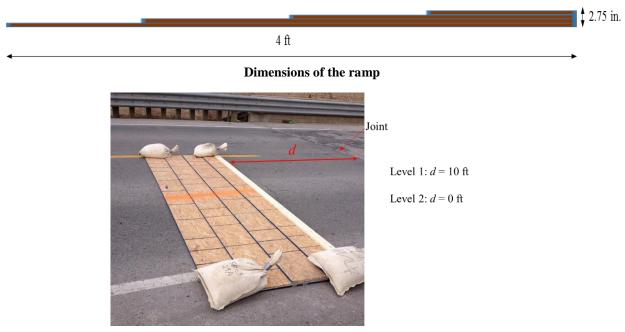
Level 1 and Level 2 ramp distances from joint Figure 3.1 Entrance conditions
