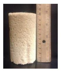
Figure 6. Cemented sand after MICP treatment
