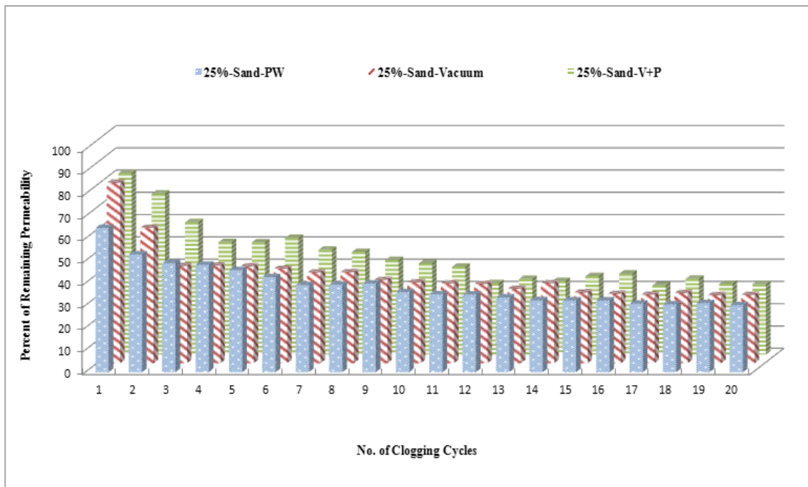
Figure 52. Sand specimens, 25 percent porosity, cleaned by three rehabilitation methods
