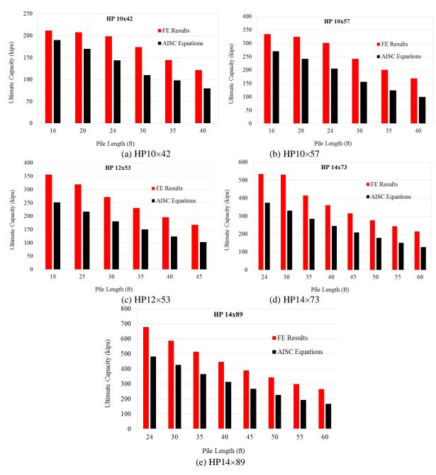
Figure 4.6 Comparisons between the pile strengths derived from the AISC equations and FE results – eccentric loads/no concrete encasement
