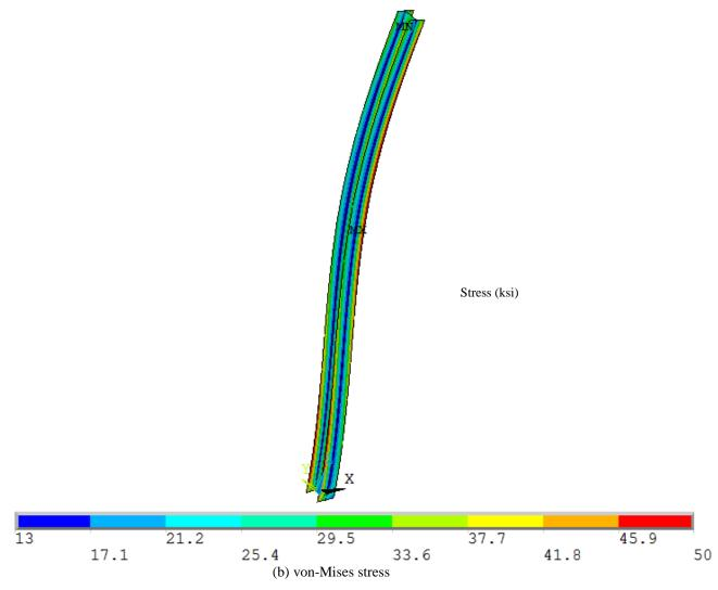
Figure 3.6 Stress in the FE model at failure
