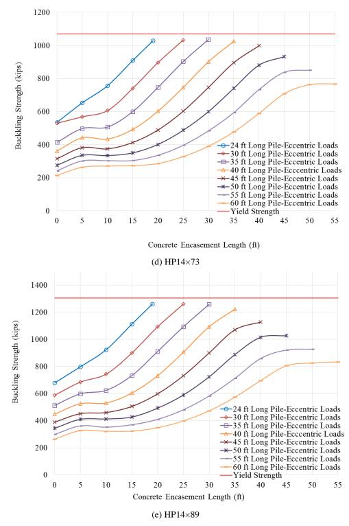
Figure 4.4 Buckling strength of steel H-piles with different concrete encasement lengths under eccentric loads
