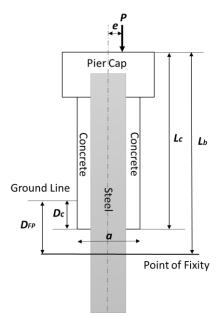
Figure 4.2 Important parameters for the pile bent
