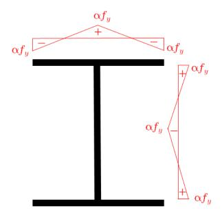
Figure 3.3 Bilinear residual stress distribution
