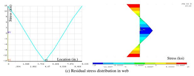
Figure 3.5 Residual stress in flanges and web of the pile
