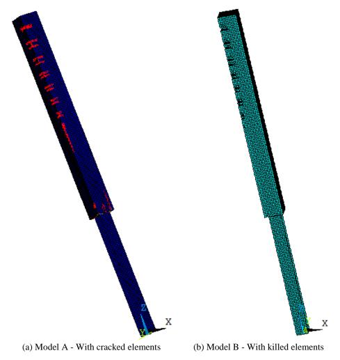
Figure 3.12 FE model with different crack modeling techniques
