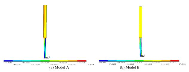
Figure 3.13 Z-stress contours of different FE models
