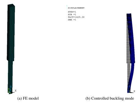
Figure 3.8 FE model and controlled buckling mode of the example pile with concrete encasement
