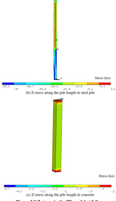
Figure 3.9 Z-stress in the FE model at failure
