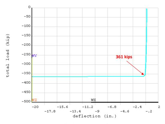
Figure 3.7 Load-deflection relationship for the FE model
