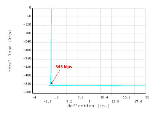
Figure 3.10 Load-deflection relationship for the FE model
