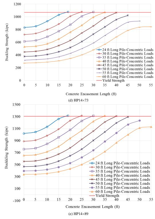
Figure 4.3 Buckling strength of steel H-piles with different concrete encasement lengths under concentric loads
