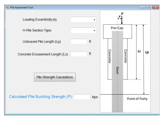
Figure 4.8 Graphical user interface of the pile assessment tool
