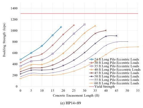
Figure 4.7 Calibrated buckling strength of steel H-piles with different concrete encasement lengths under eccentric loads
