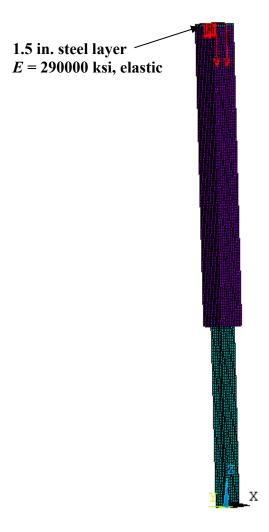
Figure 3.11 FE model with eccentric loads
