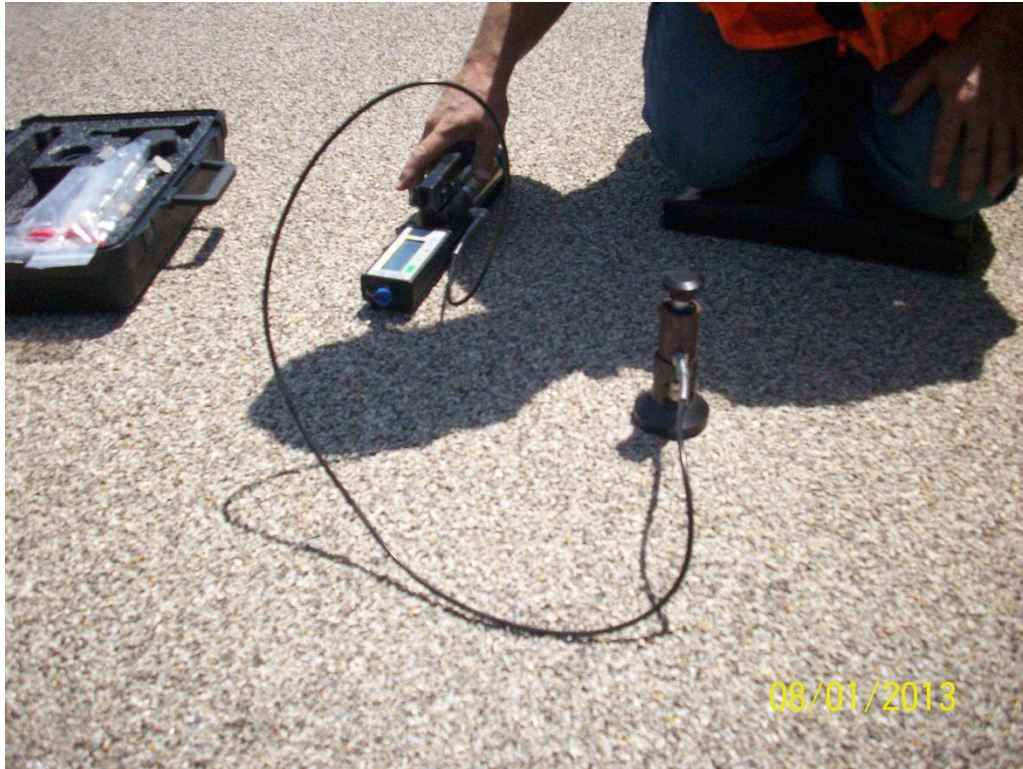
Figure 35. Tensile tests on Johnson County deck surface
