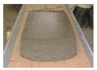
Test section of SCC extruded from mini-paver
