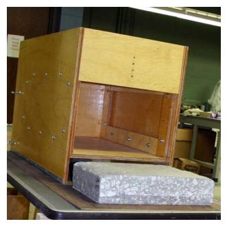
Mini-paver with section of SCC pavement slab
