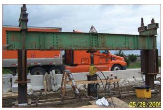
Completed static load test frame
