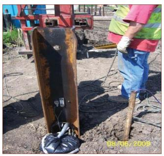
Pore water and lateral earth pressure measurement
