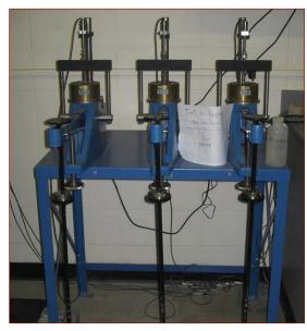
Laboratory soil tests (consolidation test)
