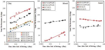
Measured pile setup using PDA and CAPWAP
