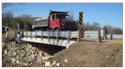
Load testing the completed, single-span, 50 ft (center to center of supports), Buena Vista County IBRD bridge
