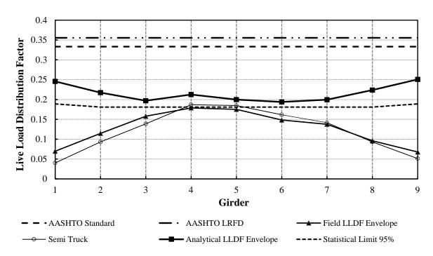
Figure B-40. LLDFs for Steel-Timber Bridge 5
