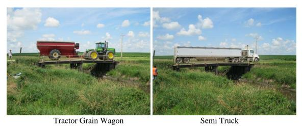
Figure A-20. Farm vehicles used for field testing
