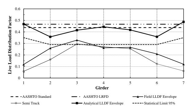
Figure B-24. LLDFs for Steel-Timber Bridge 3
