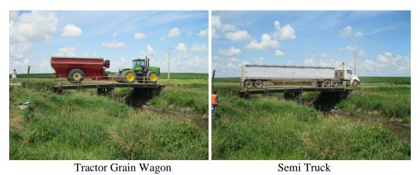
Figure C-20. Farm vehicles used for field testing
