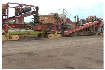
Figure 2. Mobile on-site crushing equipment (photo courtesy of Kevin Merryman, Iowa DOT)
