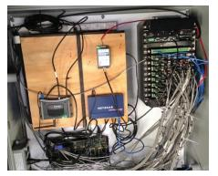
Typical field installation of SHM equipment
