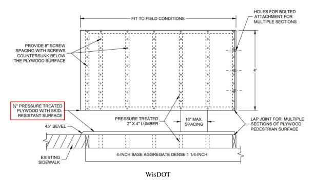
Figure 14. WisDOT standard detail drawing for temporary plywood pedestrian surfaces
