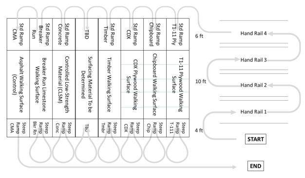
Figure 17. Conceptual plan view of Pedestrian Test Track, showing test lanes and direction of pedestrian circulation
