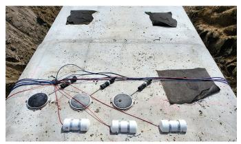
Crawford County pressure cells and strain gauges for one of three culvert sections
