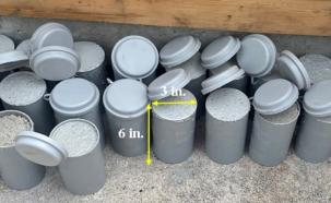
3 in. diameter × 6 in. UHPC cylinders
