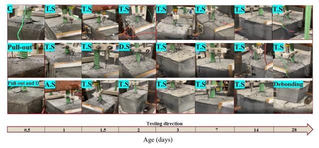
AS=all direction splitting, C=conical surface, DS=diagonal splitting, TS=transverse splitting
