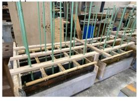
**Installing 0.5 in. divider to form discontinuous samples**
