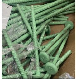
No.6 Epoxy-coated deformed rebars
