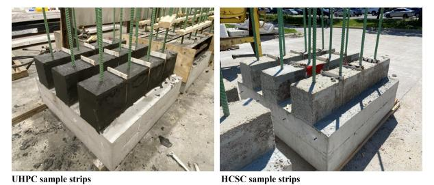
Figure 16. Completed UHPC and HCSC strips
