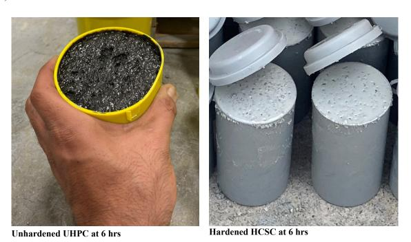
Figure 20. UHPC and HCSC materials at 6 hrs.
