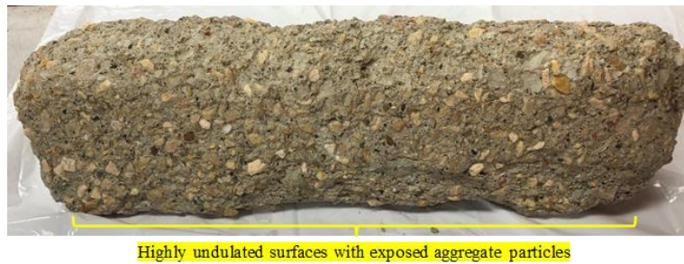
(c) Surfaces with aggregate particles exposed on the surfaces after 108 freeze-thaw cycles
