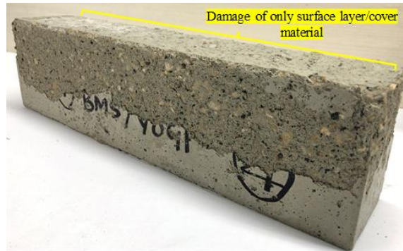
(b) More than 40% to 50% degradation of only surface layer material after 72 cycles
