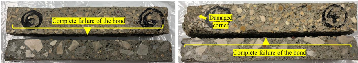
(c) Complete failure at the LMC-VE-substrate interface (separation of overlay and substrate) after 144 freeze-thaw cycles
