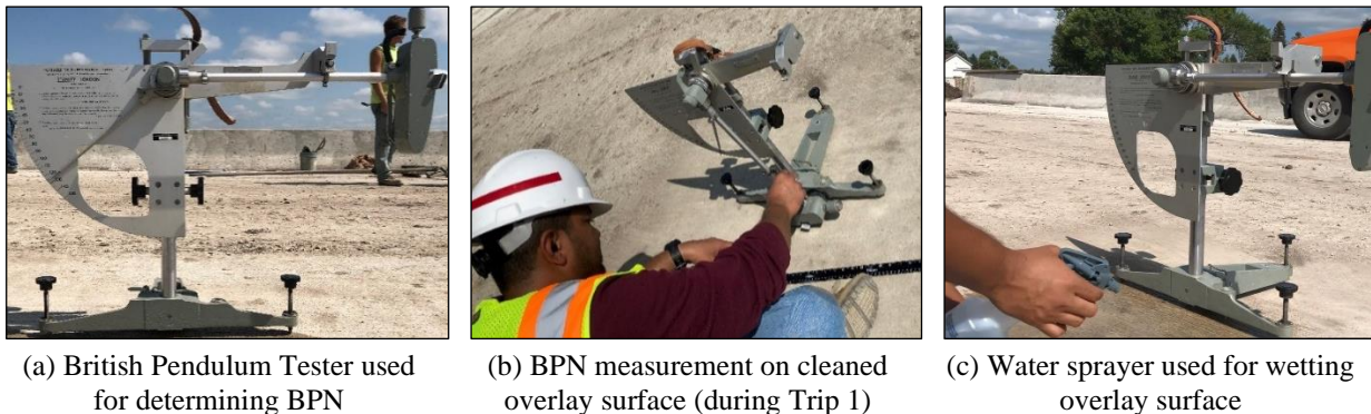
Figure 5.2. British Pendulum Tester used for measuring BPN
