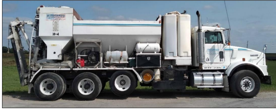
(a) Mobile mixing truck
