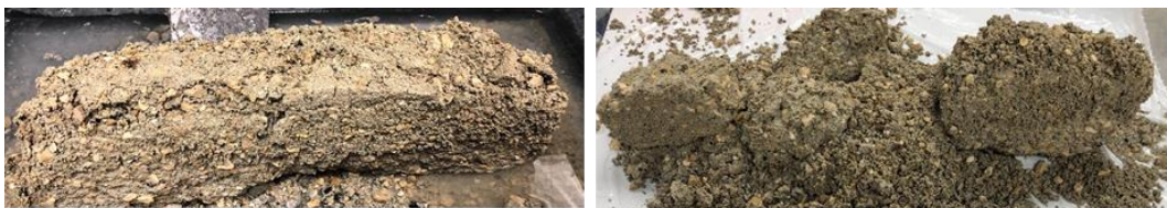
(d) Completely deteriorated beams after 144 freeze-thaw cycles
