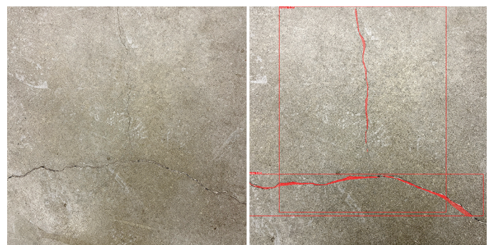
Concrete crack image (left) before and (right) after automated defect detection
