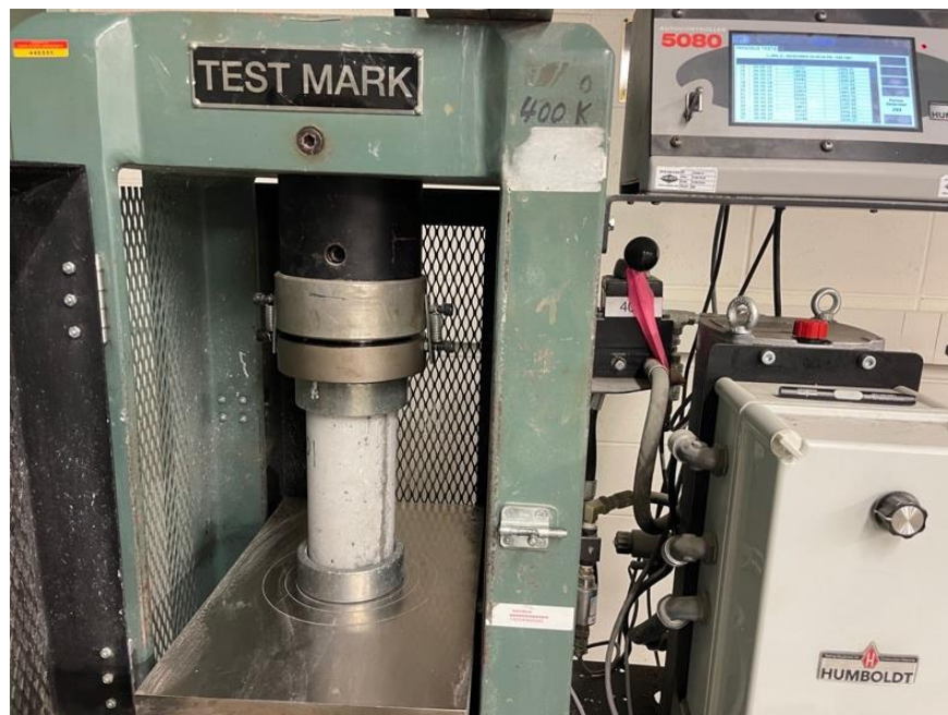
Figure 3.5. Test setup for concrete compressive strength
