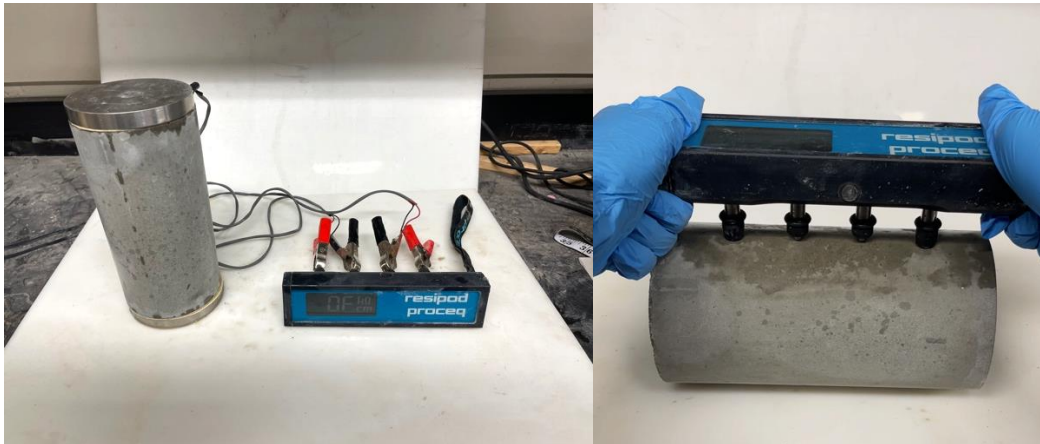
Figure 3.6. Measurement of bulk resistivity (left) and surface resistivity (right)
