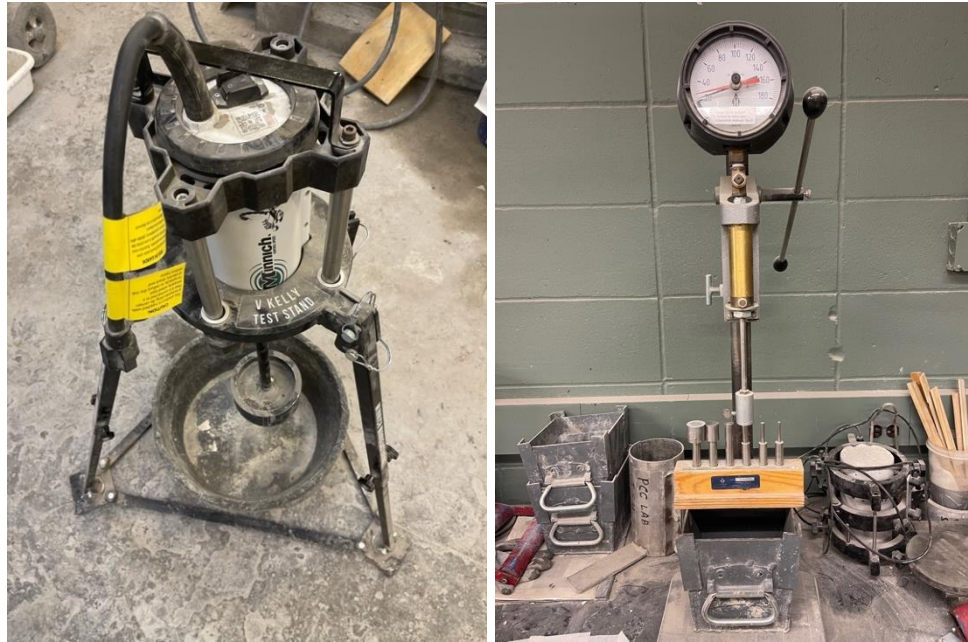
Figure 3.4. Test setup for fresh concrete: (a) VKelly, (b) penetrometer device
